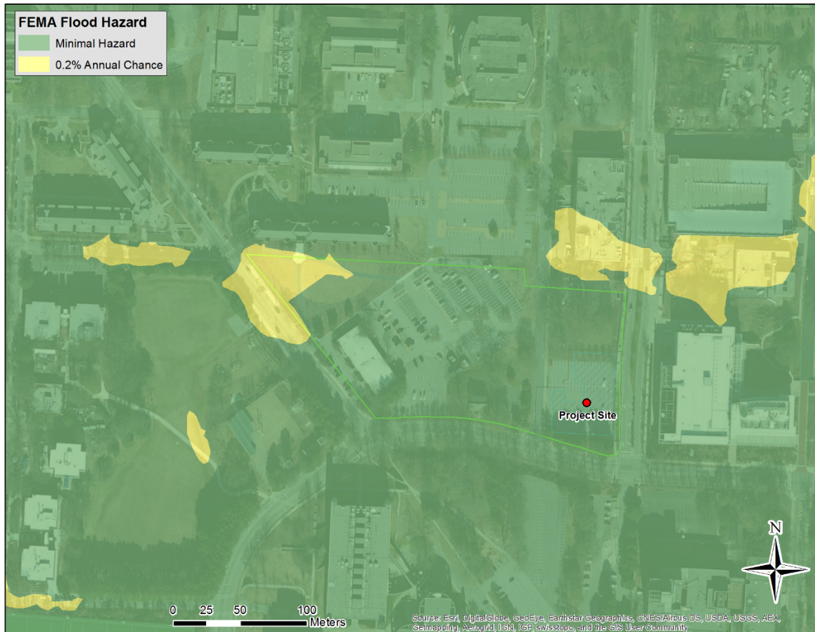
Figure 2.8a: FEMA classification of the flooding hazard in the vicinity of the proposed building site
